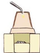
An alternate approach is to juryrig a furnace from a flower pot. Line the terra cotta pot with aluminum foil to reflect the heat, and find a way to prop a jeweler's torch so that its flame is directed into the chamber. This method reaches around 1500° F (815° C), which is good for several versions of metal clay. It is practical for 10-minute firings; something that isn't comfortable when you're holding the torch the whole time.
